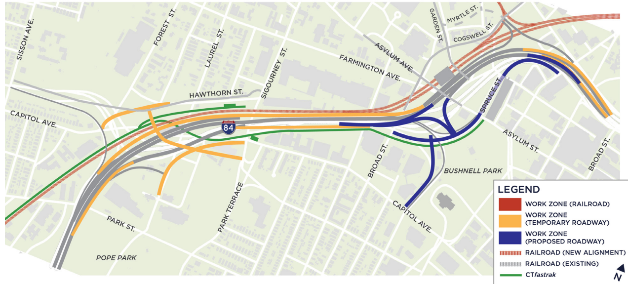
Phase 3 of construction could create better connections between Hartford's neighborhoods with Downtown and Bushnell Park. Temporary roadways are shown in yellow. Proposed permanent roadways are in blue.
