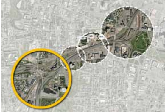
The Sisson Avenue ramps occupy an excessively large land area, having originally been designed to provide connection to a future highway to the north that was never constructed.
